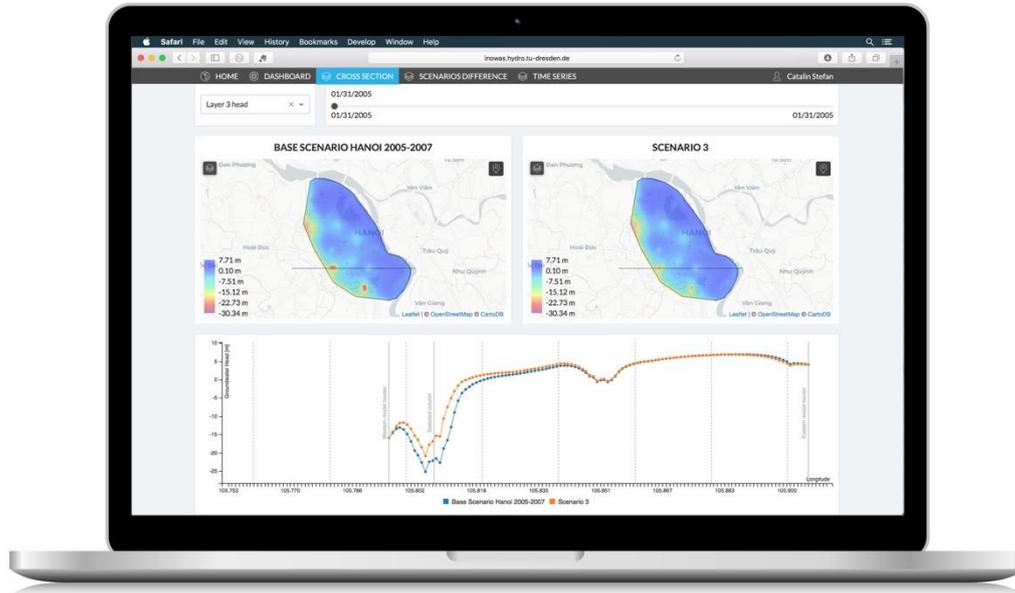
Screenshot of MODFLOW-based groundwater numerical modeling tool using the free, open source INOWAS platform
